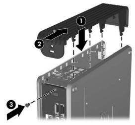
Figure 2-3 Replacing the secure compartment cover
